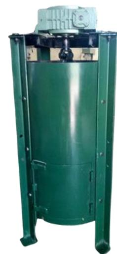
Fruits go through a digester, to then be mechanically pressed in order to extract oil from the pulp.
